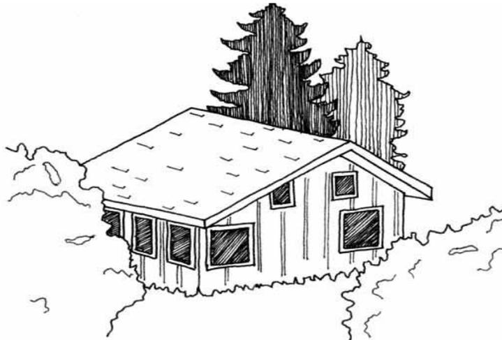
Continuous glass on less visible portion of structure
