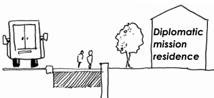
Sidewalks and curbs act as physical barriers to prevent unauthorised vehicles to approach the diplomatic mission premises
